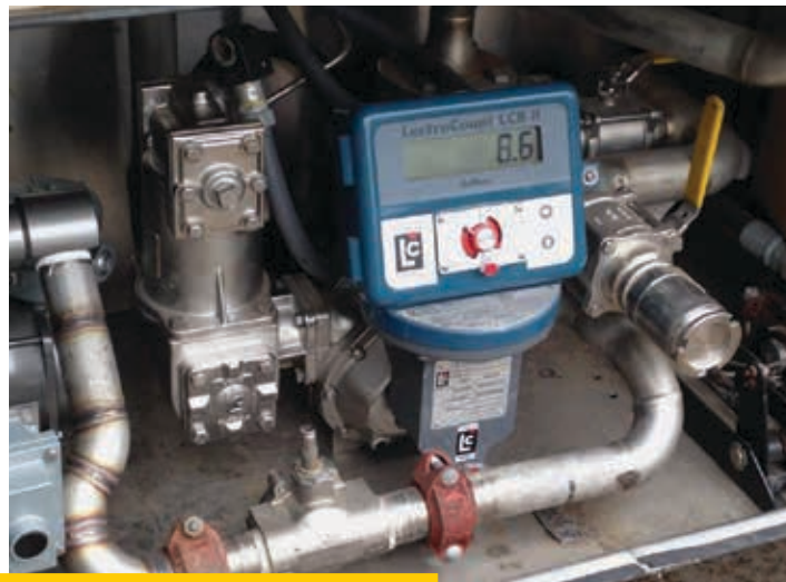
DEF Positive Displacement Flowmeter System
