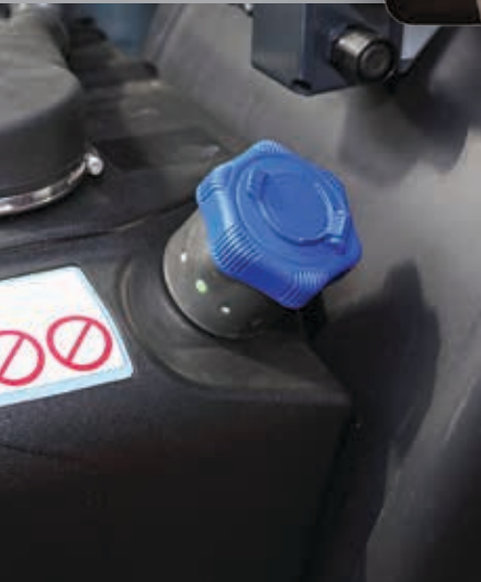
LC Optical Sensor that is placed upstream to detect air before it is introduced into the PD Flowmeter System. If air is detected the sensor will stop the flow of product and shut the valves.
