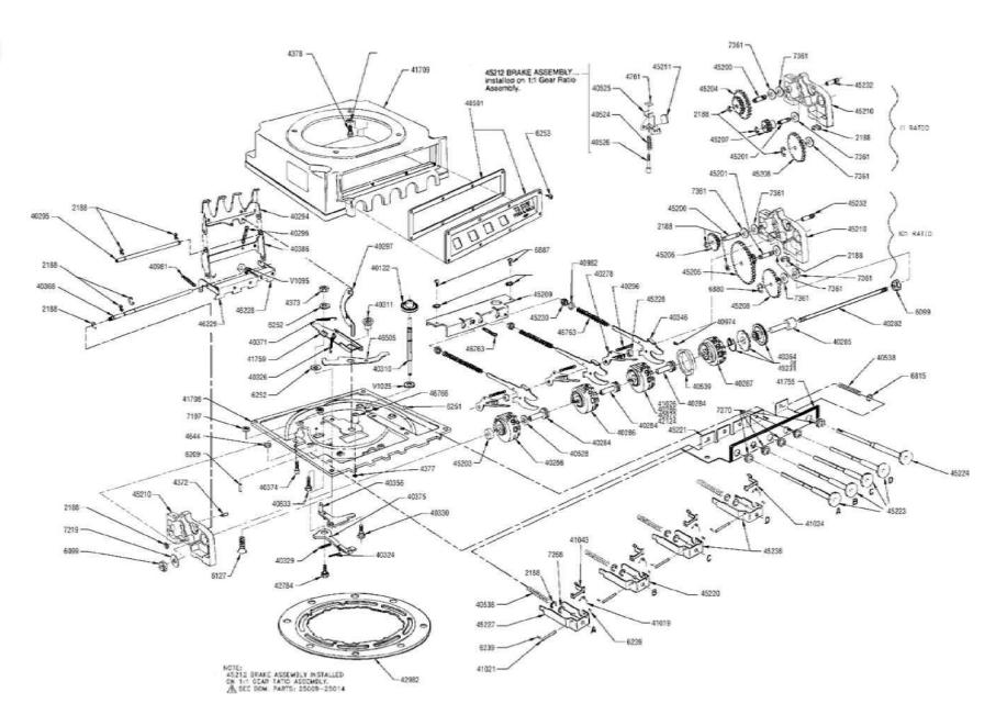
The same parts are used for all model Presets, except (1)the number wheels 40286, 40972, 41026 and 42124 (see model description, pages 3 and 4) and (2) the gears 45204, 45205, 45206, 45207, 45208, that are part of the side frame and gear Assemblies (see description in listing below, Part Nos. 45213 and 45214).
