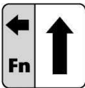
Arrow Button to scroll the pointer up the left side of the display
