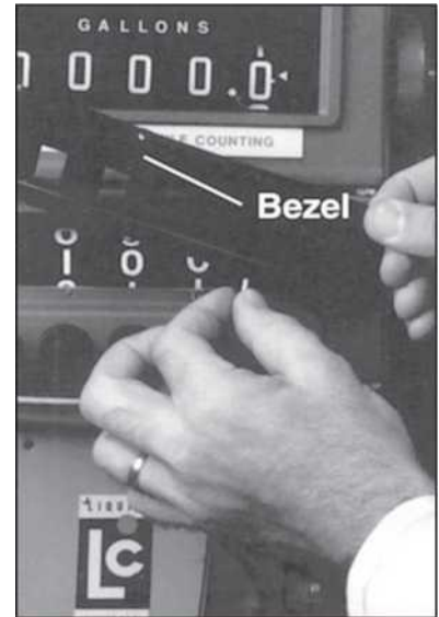
Figure 13a: Bezel Removal
