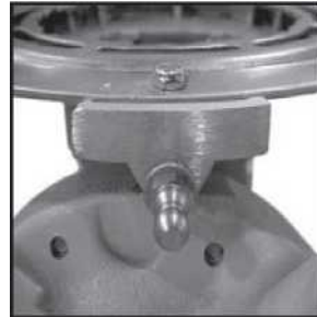
Figure 17a: Ball Joint
