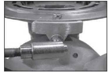
Figure 6b: Linkage Attached to Ball Joint
