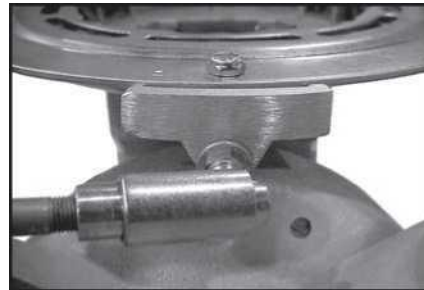
Figure 17b: Linkage Attached to Ball Joint
