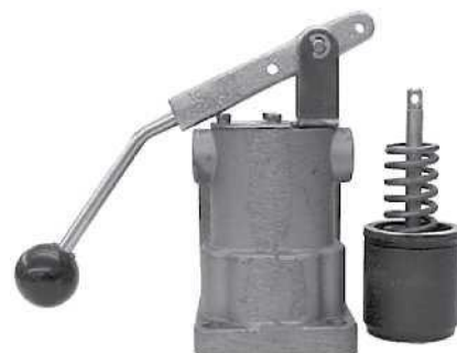
Figure 17e: Piston Assembly Removed
