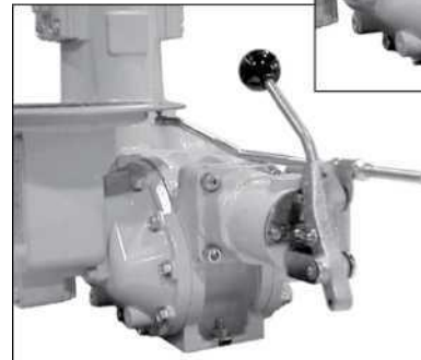
Figure 8b: Rear Facing Outlet
