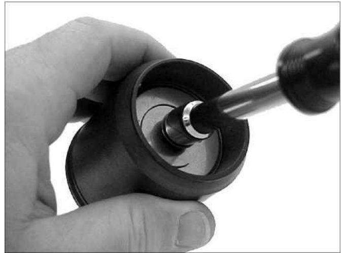
Figure 18a: Piston Assembly
